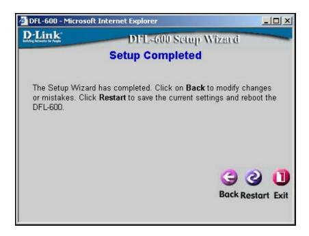
You have completed the basic setup Wizard. The configuration now needs to be entered into the DFL-600's non-volatile RAM. Clicking **Restart** will save the configuration to non-volatile RAM and restart the router.
